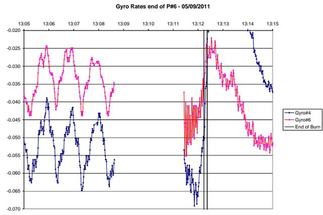
**Figure 9. Gyros output at the end of the final burn**
