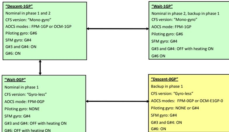
**Figure 5. ACS configurations during descent**
