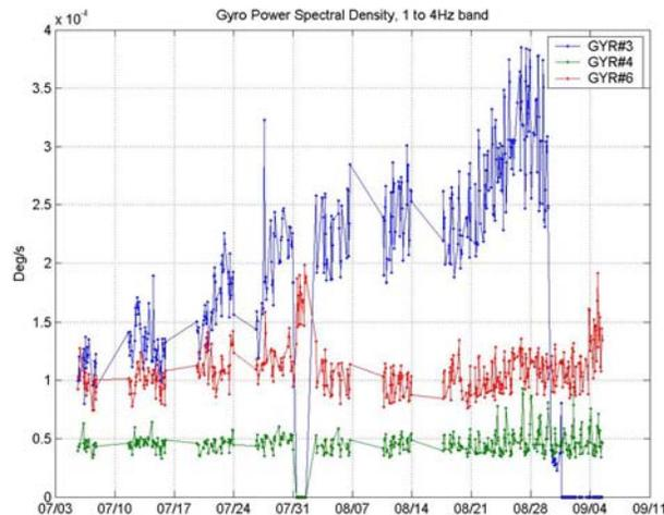
**Figure 6. PSD 1-4 of gyro 3, 4, and 6 throughout disposal**
