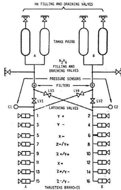
Figure 3. Diagram of ERS 2 propulsion
